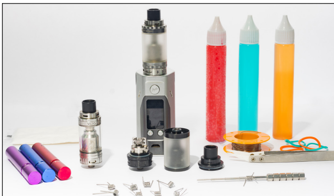
(Top) JUULs or similar products come in different colors and look like a flash drive. (Bottom) The different parts of e-cigarettes include heating coils and flavoring liquids.
